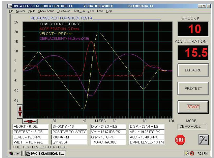
automatically resizes for use with any monitor. No ISA slots required!
